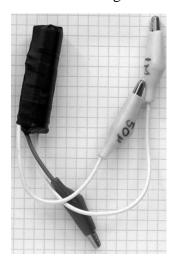
To use – simply connect –ve to the negative terminal and try a first test with the 50uA lead.
